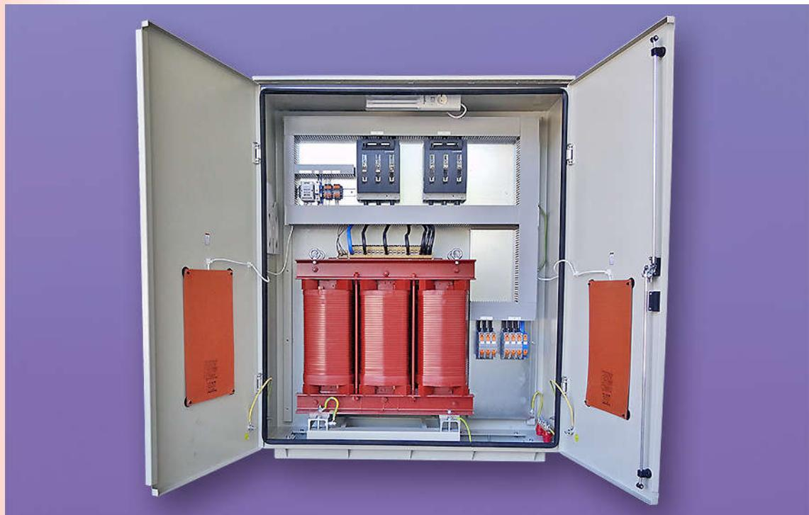
**Isolation Transformer Cabinet, type: EK OTR is used for power supply Railway points heating control cabinet, type: EK URO. The input of the EK OTR is connected to the Elektro-distribution network. The output of the EK OTR is connected to the input of the Railway points heating control cabinet (EK URO). Railway points heating system has an insulated low voltage network (IT system - all active conductors are isolated from earth) with permanent insulation resistance control.**
