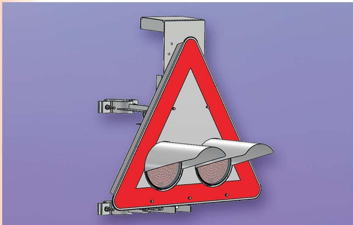
**Level crossing (ŽCPR) is a place where a road crosses railway track. To avoid accidents, these places are assured on various ways. One way is to use light traffic sign. EK LS-ŽCPR is a traffic light sign used on level crossings. To participants in road traffic, it signals the arrival of a railway vehicle. It is consisted of two lamps, EK SLZCP-180, derived in LED technology.**
