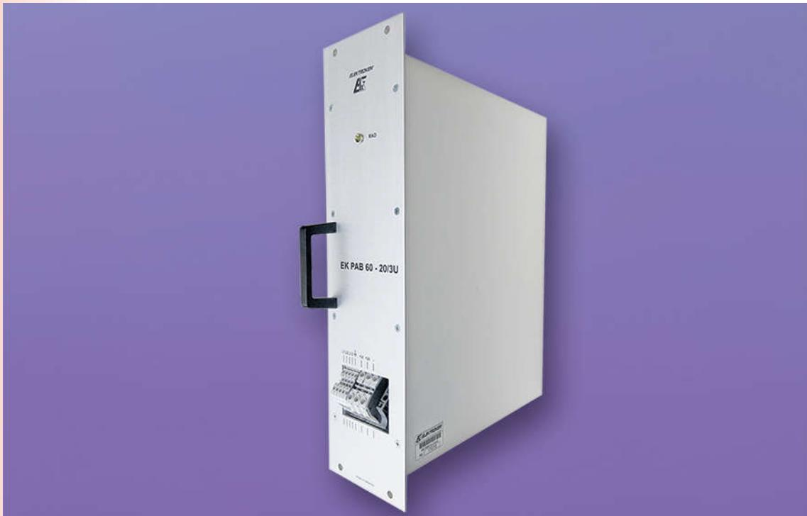
**Rectifier - Charger, type: EK PAB 60- 20/3U is designed for charging lead-acid batteries with rated voltage of 60 V. The charger is also used for powering the consumer on an equal 60 V voltage, with a charged battery as well as without a charged battery. The nominal permanent output current is 20 A. In the case of the need of larger currents, the rectifier-charger supports the connection to parallel operation with one or more rectifier-chargers of the same type tag.**
