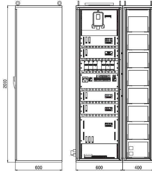
The power supply equipment BN-SP-2000 is purposed for power supplying signal and safety railway station equipment. It is consisted of a set of voltage sources whose voltages are adjusted to a specific load requirements.
