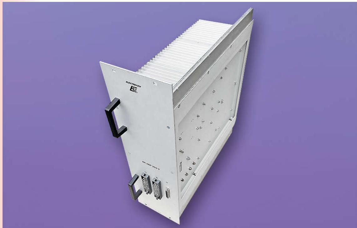
The purpose of the Electronic Bypass EK ABP 25/3 V is to measure and transmit to the output terminals of the correct three-phase sinusoidal voltage (3x230 / 400V, N, PE) which is coming from the inverter modules and the distribution network of the EK BNSP 20000 Power Supply System. Depending on informations of the correctness and priority of this voltage The Central Control Unit sends control impulses and turns on and off the thyristor switches in the electronic bypass module.
