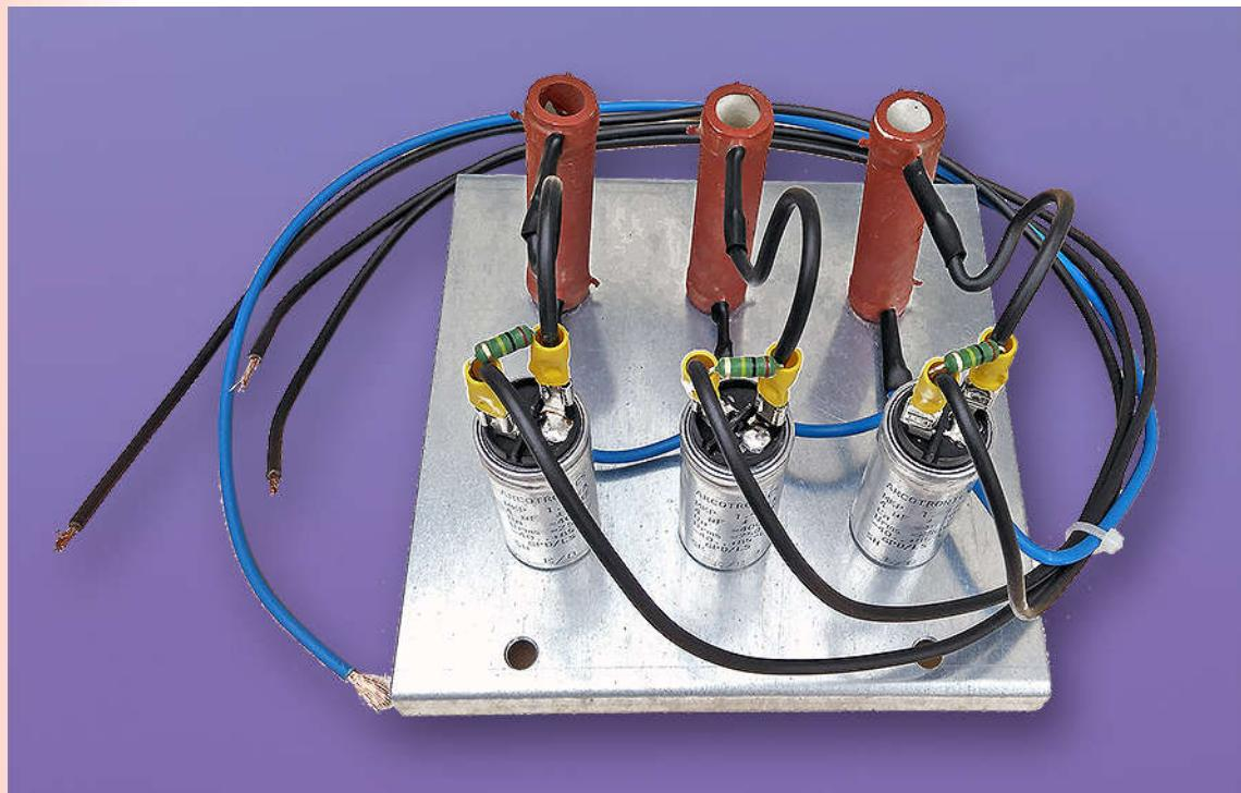
**The EK MNT BNSP-20000 Minimum Load Module is designed to ensure minimum system power while the system is unloaded. Also, the EK MNT BNSP-20000 is used to dissipate overvoltage which is generated unloaded system.**
