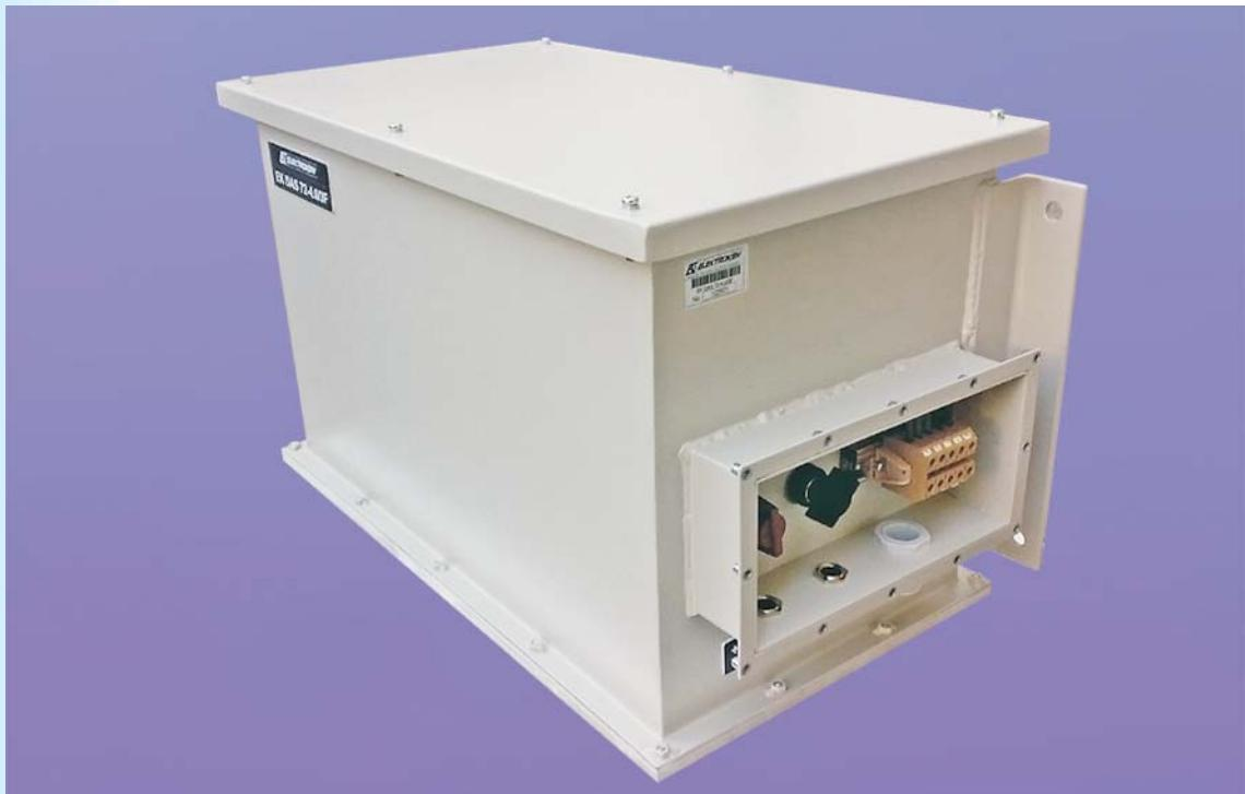
**Electronic DC/AC inverter EKDAS 72-4.0/3F powered by energy from the battery pack three phase air conditioning compressor and single-phase heater oil on the locomotive. DC/AC converter at its output generates three-phase AC voltage (3x400V, 50 Hz), galvanically separated from the battery, the sine wave with a distortion factor of less than 2%. Input voltage converter is a DC voltage of the battery pack, with the appropriate charger, rated voltage of 72V.**
